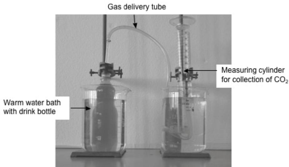
The volume of gas was measured, at 28°C and 102.4 kPa, and recorded when no further change in the height of water in the upturned measuring cylinder was observed. This procedure was carried out four times. The results are shown in the table below.
